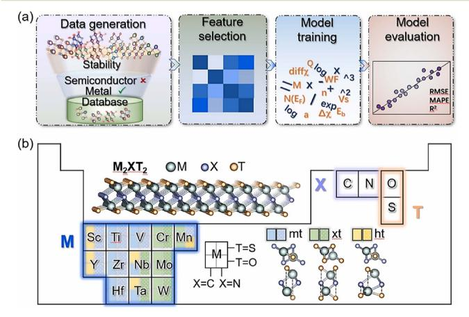
Fig. 6 (a) The process flow of ML is illustrated in the workflow diagram. (b) The distribution of elements and structures within  $M_2XT_2$  (T = bare, O, S). Reproduced with permission from ref. 11. Copyright 2023 Elsevier.
