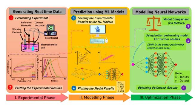
Fig. 3 A schematic representation of utilizing ML models to forecast electrochemical characteristics in supercapacitor electrodes with MXene and graphene nanoplatelets. Reproduced with permission from ref. 14. Copyright 2024 Elsevier.
