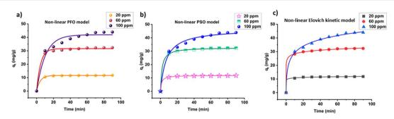
Fig. 12 Non-linear fitting of pseudo first order (a); non-linear fitting of pseudo second order (b) and non-linear fitting of Elovich (c) kinetic model for the adsorption of Malachite Green on ACFCeP composite (pH = 7, dose = 50 mg, time = 90 min).
