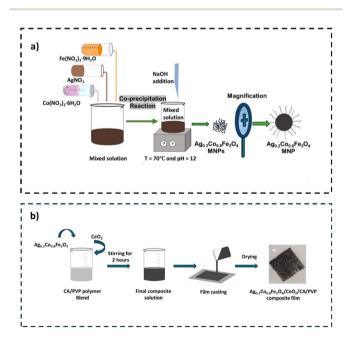
Scheme 1 Preparation of the Aq-doped cobalt ferrite (a); preparation of the Ag<sub>0.2</sub>Co<sub>0.8</sub>Fe<sub>2</sub>O<sub>4</sub>/CeO<sub>2</sub>/CA/PVP (ACFCeP) composite film (b).
