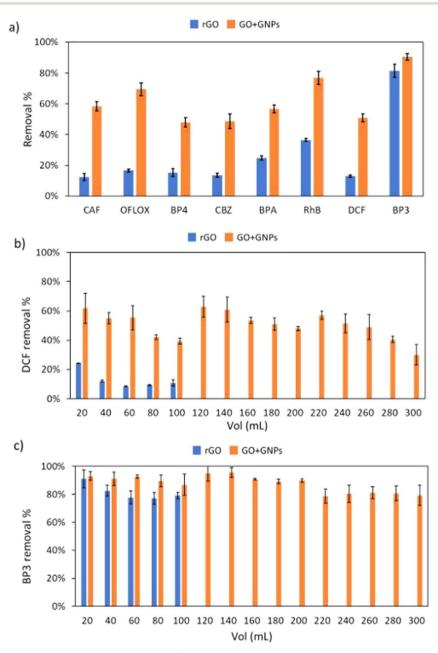
Fig. 7 (a) Average removal of a mixture of eight ECs (0.5 mg L $^{-1}$  each in tap water,  $V_{\text{tot}} = 100$  mL, flow rate = 2.5 mL min $^{-1}$ ) by aerogels of rGO (blue) and GO + GNPs (orange); removal of (b) diclofenac (DCF) and (c) benzophenone-3 (BP3) (0.5 mg L $^{-1}$  each in tap water,  $V_{\text{tot}} = 300$  mL, flow rate = 2.5 mL min $^{-1}$ ).
