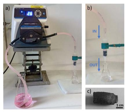
Fig. 6 The photographs of (a and b) the experimental set-up used to test (c) aerogels under flow conditions.
