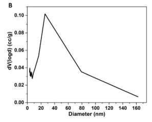
Fig. 3 (A) Pore characterisation of the GO + GNP aerogel. The nitrogen adsorption—desorption isotherm of the aerogel is shown. The BET surface area and nitrogen adsorption—desorption isotherms were measured using the analysis program of the micropore physio-/chemisorption analyser. (B) Barrett—Joyner—Halenda (BJH) pore size distribution curve of the examined aerogel.
