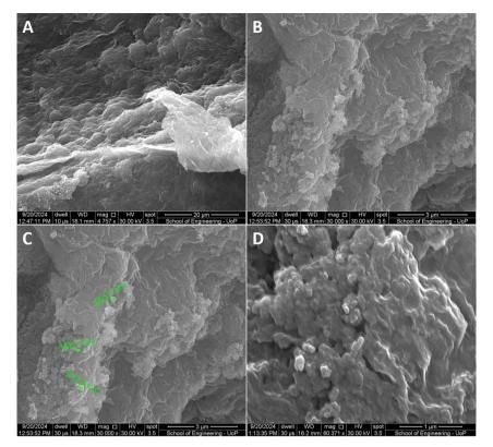
Fig. 5 Several SEM images of the as-prepared GO + GNP aerogels at different scale bars (A, B and D). In (C), the size of some GNP crystals is measured and depicted.
