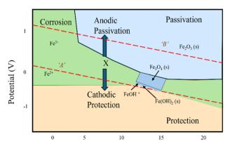
Fig. 3 Pourbaix diagram for steel. 15
