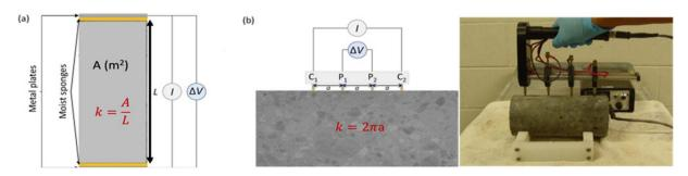
Fig. 9 A schematic diagram of resistivity measurement (a) uniaxial configuration for bulk resistivity, (b) Wenner configuration schematic diagram (left), experimental setup for Wenner configuration (right). 68,69
