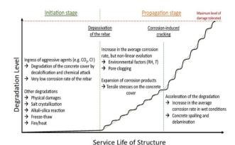
Fig. 1 Schematic representation of the corrosion progression in RC, based on the Tuutti model, with consideration for the service life. 7.9.12
