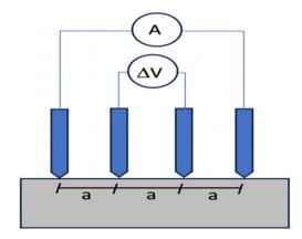
Fig. 10 Concrete resistivity measurement by four electrodes.83
