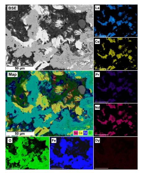
Fig. 14 SEM-BSE image of siderite grain being replaced with kozoite in PAAS solution at 165 °C after 24 hours and EDS maps showing the almost heterogenous distribution of REE.
