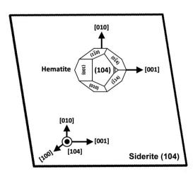
Fig. 8 Schematic diagram showing the epitaxial relationship between hematite and siderite crystals.
