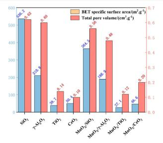
Fig. 7 BET data of different carriers and MnO<sub>x</sub>/WO<sub>y</sub> catalysts.
