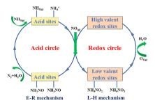
Fig. 9 Schematic diagram of NH<sub>3</sub>-SCR reaction pathway on metal oxide and zeolite catalysts (reproduced from ref. 29 with permission from ACS Publications).
