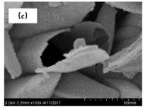
Fig. 6 The SEM images of  $MnO_X$ - $CeO_2$  hollow nanotube: (a-c). (Reprinted from ref. 57. Copyright 2018, with permission from Elsevier).
