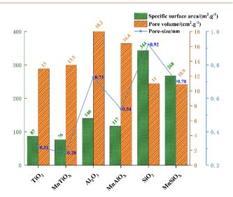
Fig. 8 BET data of different carriers and MnO<sub>2</sub>/WO<sub>v</sub> catalysts.
