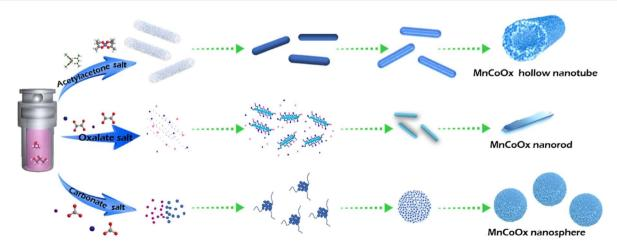
Fig. 5 The schematic illustration of the formation of the hollow nanotube, nanorod, and nanosphere of  $MnCoO_X$  oxides (eeprinted from ref. 53. Copyright 2021, with permission from Elsevier).
