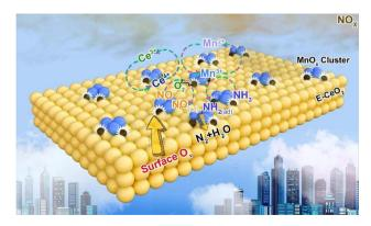
Fig. 12 Schematic reaction mechanism of MnO<sub>X</sub>-CeO<sub>2</sub> catalyst synergistic effect (reprinted from ref. 114. Copyright 2023, with permission from Elsevier).
