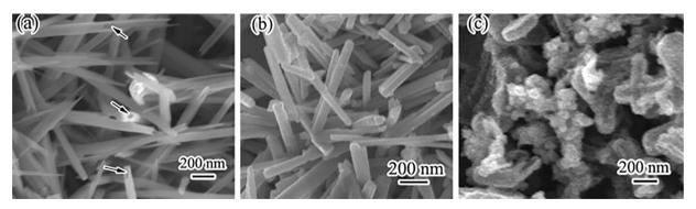
Fig. 3 The SEM images of the  $MnO_2$  catalysts (a) nanotubes; (b) nanorods; (c) nanoparticles (reprinted from ref. 35. Copyright 2011, with permission from Elsevier).
