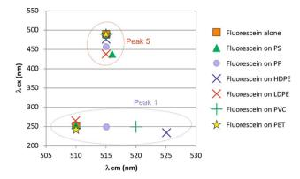
Fig. 6 Molecular fluorescence excitation  $(\lambda_{ex})$  and emission  $(\lambda_{em})$  wavelengths of peaks observed for fluorescein alone and that adsorbed on the nanoplastics.
