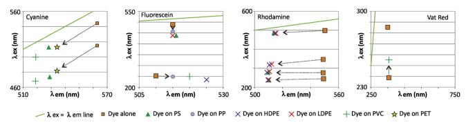
Fig. 12 Direction of variation of the shift of fluorescence peaks of dyes after adsorption on nanoparticles
