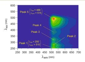
Fig. 5  $\,$  3D fluorescence spectra of fluorescein in solution (10 mg L $^{-1}$ ), using arbitrary units for intensity.
