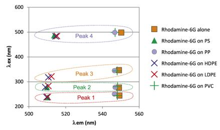
Fig. 9 Molecular fluorescence excitation ( $\lambda_{ex}$ ) and emission ( $\lambda_{em}$ ) wavelengths of peaks observed for rhodamine-6G alone and that adsorbed on the nanoplastics.
