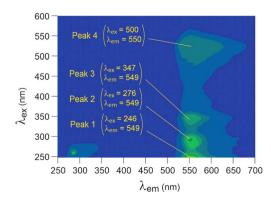
Fig. 8 3D fluorescence spectra of rhodamine-6G in solution (10 mg  $\rm L^{-1}$ ), using arbitrary units for intensity.
