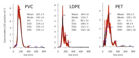
Fig. 1 NTA size distributions of nanoplastics in suspension. Statistical values are given in nm.
