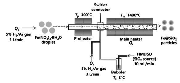
Fig. 2 Experimental setup of synthesizing Fe@SiO<sub>2</sub> particles
