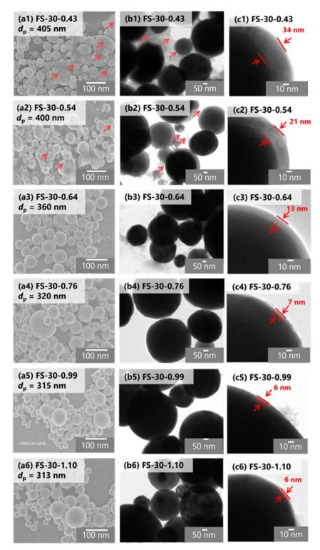
Fig. 5 The effect of the number of cores on the morphology of Fe@SiO $_2$  particles. (a) SEM and TEM images of Fe@SiO $_2$  particles at a different number of cores: (1)  $0.43 \times 10^6$ , (2)  $0.54 \times 10^6$ , (3)  $0.64 \times 10^6$ , (4)  $0.76 \times 10^6$ , (5)  $0.99 \times 10^6$  and (6)  $1.10 \times 10^6$  cores per cm $^3$  carrier gas at (b) low magnification and (c) high magnification.
