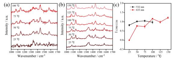
Fig. 5 Temperature-dependent SERS spectra of the plasmon-induced photocatalytic reaction of 4-NTP at high temperatures with 532 nm (a) and 633 nm (b) excitation, respectively,  $t_{aca} = 60$  s. (c) intensity ratio of 1390 cm<sup>-1</sup>/1336 cm<sup>-1</sup> referring to [DMAB]/[4-NTP] as a function of temperature at 532 nm (black) and 633 nm (red) ( $P_{532 \text{ nm}} = 1.05 \mu\text{W}$ ,  $P_{633 \text{ nm}} = 7.8 \mu\text{W}$ ).
