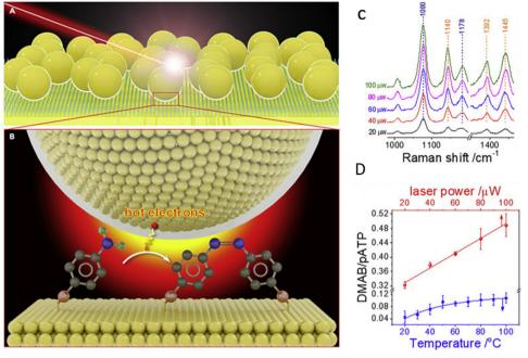
Fig. 18 (a) Scheme of in situ SERS study on the interfacial hot electron transfer in the photocatalytic conversion of p-aminothiophenol (p-ATP) to dimercaptoazobenzene (DMAB). (b) SERS spectra of the conversion of p-ATP catalyzed by Au NPs at different laser power excitations. (c) The relative intensity of DMAB to p-ATP bands with different incident laser powers. The figure is adapted from ref. 582 with permission from Springer, Copyright 2020.
