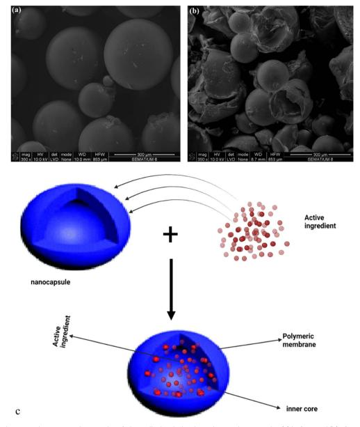
Fig. 5 Scanning electron microscopy micrographs of citronella-loaded polyurethane microcapsules (a) before and (b) after mechanical stress. Reproduced from ref. 50 with permission from Elsevier, copyright 2016. (c) Schematic representation of the structure and drug loading processes for micro/nanocapsules (created with BioRender).
