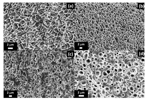
Fig. 9 SEM micrographs showing the effect of insect repellent type and concentration on the structure of the internal microprorous region of extruded LLDPE strands. (a) 20 wt% DEET, (b) 30 wt% DEET, (c) 20 wt% icaridin, and (d) 30 wt% icaridin. Reproduced from ref. 15 with permission from Elsevier, copyright 2019.
