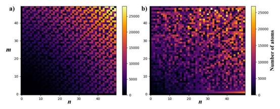
Fig. 7 Plot of the number of atoms corresponding to each (n, m) pair for n, m < 50 for (a) CNTs and (b)PNTs. Color represents the number of atoms in the CNT supercells and is plotted in a plane where the x and y axes represent the chiral indices n and m, respectively.
