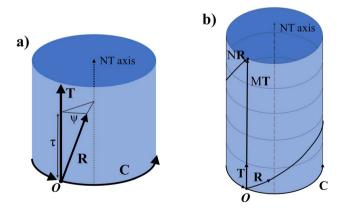
Fig. 3 (a) Schematics of a NT unit cell showing the folded nanoribbon and its now circular chiral vector C along with the translational vector T parallel to the NT axis. The symmetry vector R is shown with its component in the T direction  $\tau$  and the rotation around the NT axis  $\psi$ . (b) M nanotube unit cells joined together through the shared NT axis. The R vector is shown extended N times so that it wraps around the NT, ending up on a point equivalent to the origin O.
