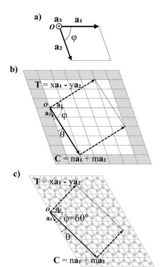
Fig. 1 (a) Unit cell of an arbitrary 2D material.  $a_1$ ,  $a_2$  and  $a_3$  are the vectors of the unit cell.  $\varphi$  is the angle formed between  $a_1$  and  $a_2$ . (b) Lattice of a general 2D material with the nanoribbon delimited by the chiral vector  $\mathbf{C}$  and the translational vector  $\mathbf{T}$ . (c) Graphene lattice with a nanoribbon defined by  $\mathbf{C}$  and  $\mathbf{T}$ .
