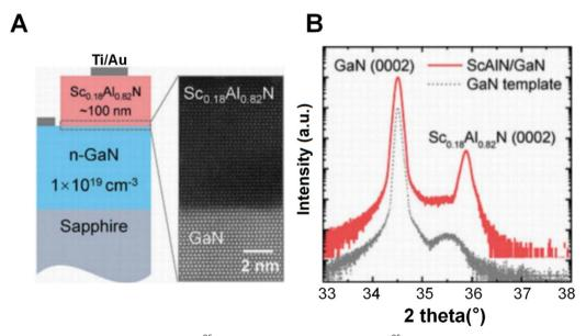
Fig. 2 (A) ScAlN-GaN thin film structure grown on GaN. 95 (B) XRD results of ScAlN/GaN films. 95
