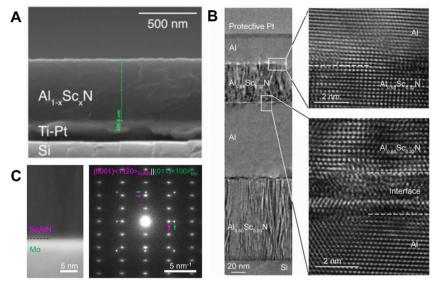
Fig. 1 (A) ScAIN-Pt thin film structure grown on Ti-Pt substrates. 91 (B) Film structure with Al and ScAIN mutually superposed. 45 (C) Structure of ScAIN-Mo thin films grown on Mo. 46
