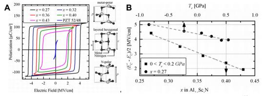
Fig. 4 (A) Ferroelectric Sc<sub>x</sub>Al<sub>1-x</sub>N with Sc contents of 0.27, 0.32, 0.36, 0.46, 0.43 and 0.43 and PZT is the P-E ring of Sc<sub>x</sub>Al<sub>1-x</sub>N. 105 (B) Dependence of the average stress field on the residual stress Tr and Sc content of  $Al_{1-x}Sc_xN$  films. Sc content and Tr content vary independently. <sup>105</sup>
