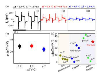
Fig. 4 (a) Pyroelectric response along b-axis under temporal change in temperature of (i) 6.7 °C ( $\Delta T = 1.8$  °C s<sup>-1</sup>), (ii) and 1.6 °C ( $\Delta T = 0.6$  °C s<sup>-1</sup>) (iii) 0.9 °C ( $\Delta T$  = 0.3 °C s<sup>-1</sup>), (b) pyroelectric coefficient as a function of temperature change and (c) comparison of pyroelectric coefficient in different materials (ref. 26-36).
