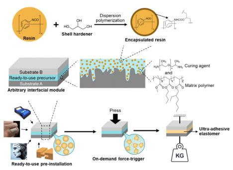
Fig. 1 Illustration of the on-demand ultra-high adhesion formation of the ready-to-use precursor and its preparation process. The resin, curing agent, and matrix polymer are MDI-prepolymer, PPG-diamine, and acrylates copolymer, respectively.
