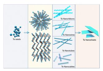
Fig. 1 Schematic of the morphological evolutions and transformations of Te nanostructures.
