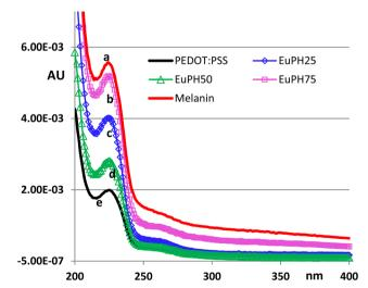
Fig. 2 UV spectra of (a) DHI-melanin, (b) EuPH75, (c) EuPH50, (d) EuPH25 and (e) PEDOT:PSS thin films on quartz. Absorbances are normalized to the thickness.
