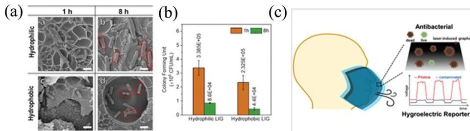
**Fig. 10** (a) Antibacterial activity of hydrophilic/hydrophobic LIG substrates: *E. coli* SEM images on hydrophilic/hydrophobic LIG substrates (2  $\mu\text{m}$  scale). (b) CFU (colony forming unit) evaluated for the two samples of LIG. (c) A schematic of the hydroelectric generator application.<sup>36</sup> Copyright © 2020 American Chemical Society.
