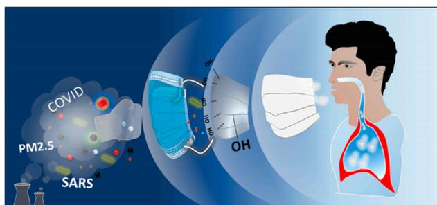
Fig. 6 Schematic of the electrospun thymol/PVB nanofibrous facemask.<sup>28</sup>
