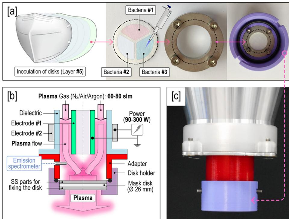
Fig. 15 (a) Extracting the  $\varnothing$  26 mm disks from KN95 masks for inoculation with *Staphylococcus aureus* ATCC29213 and *Escherichia coli*. ATCC25922. (b) Sketch of atmospheric pressure cold plasma equipment. (c) Plasma apparatus designed for treating the inoculated mask disks.<sup>87</sup>
