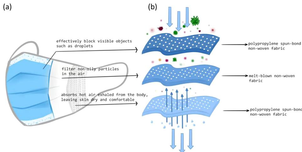
Fig. 12 Three layers in the mask structure. (a) Schematic diagram of the medical protective mask.<sup>55</sup> (b) Three-layer nonwoven mask with spun-bond and melt-blown polypropylene sheets.<sup>15</sup>
