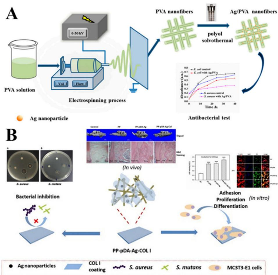
Fig. 7 (A) Schematic illustration of fabrication and the antibacterial test for Ag/PVA composite nanofibers through the electrospinning and solvothermal methods.<sup>29</sup> Copyright 2020 by the authors. (B) Triple PLGA/PCL scaffold modification including silver impregnation, collagen coating, and electrospinning significantly improves biocompatibility and antimicrobial and osteogenic properties for orofacial tissue regeneration.<sup>30</sup> Copyright 2019 American Chemical Society.
