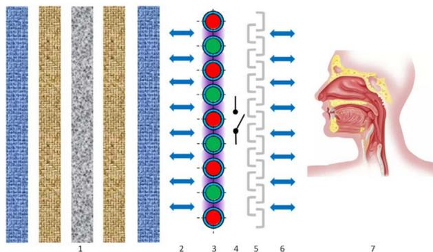
**Fig. 11** A scheme of the system. 1 is coupling layers; 2 and 6 show the bidirectional air flows; 3 is electrodes that are used to generate plasma (violet light) filling the space between the layers and the dielectric layer (5); 4 is the switching system that is able to switch on/off the plasma during the expiration/inspiration; 5 is the dielectric material to isolate the body from the electrodes; 7 is mask wearers.<sup>48</sup> Copyright © 2020 American Chemical Society.
