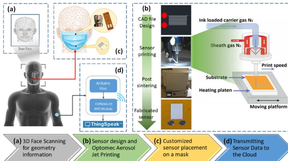
Fig. 8 The process of designing a smart mask system. (a) Obtaining 3D facial scan data and scrutinizing face geometry (b) using AJP technique printing temperature and strain sensors. (c) Schematic of the smart mask. (d) Data processing.
