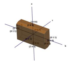
Fig. 2 Morphology diagram of the grown DMMA crystal.
