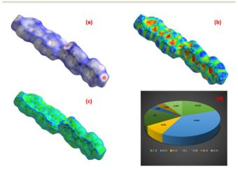
Fig. 13 Hirshfeld surface of DMMA crystal: (a)  $d_{norm}$ , (b) shape index, (c) curvedness index and (d) 2D fingerprint plot.
