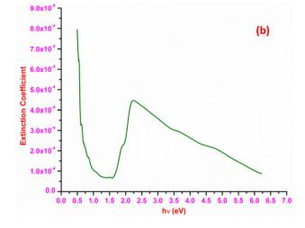
Fig. 5 (a) Bandgap and (b) extinction coefficient vs. photon energy
