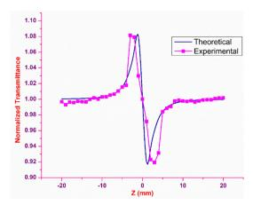
Fig. 14 Closed aperture plot of DMMA
