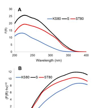
Fig. 3 Diffuse reflectance UV-Vis analysis of titanosilicate samples KS80, S and ST80. (A) Kubelka-Munk plots, (B) Tauc plots
