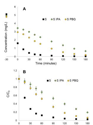
Fig. 7 Radical guenching results for the S (sunflower oil) sample, showing that IPA and PBQ scavenger compounds slow down the rate of reaction, with IPA having more of an impact than PBQ.
