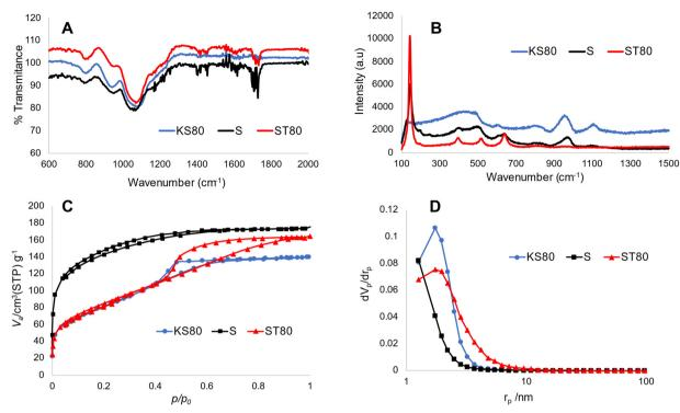
Fig. 2 Chemical and porosity characterization of titanosilicate samples KS80, S and ST80: (A) FTIR spectra, (B) Raman spectra, (C) nitrogen adsorption desorption isotherms and (D) pore size distribution (BJH) plots.
