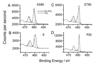
Fig. 5 Fitted high resolution Ti 2p X-ray photoelectron scans of: A-sample KS80, B-sample S, C-sample ST80 and D-P25 TiO2 standard. Fitted environments for KS80, S and ST80 were the same as those in our previous paper,<sup>29</sup> with a doublet separation of 5.72 eV. Samples KS80, S and ST80 exhibited differing ratios of TiO2 to TiO2/SiO2 components, as listed in Table 2
