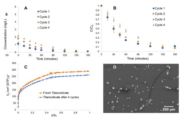
Fig. 8 Recyclability experiments on Rh B degradation with sample S as photocatalyst, over four cycles. (A) Concentration vs. time. (B) Normalized results  $(C/C_0)$  vs. time, (C) comparative nitrogen adsorption—desorption isotherms for fresh and used titanosilicate and (D) SEM of used titanosilicate, showing non-fused/broken microspheres.
