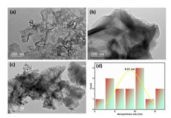
Fig. 6 TEM analysis of (a)  $g-C_3N_4$ , (b) CoCN-NaBH<sub>4</sub>, and (c) CoCN-H<sub>2</sub>. (d) NP size distribution histogram of CoCN-H<sub>2</sub>.
