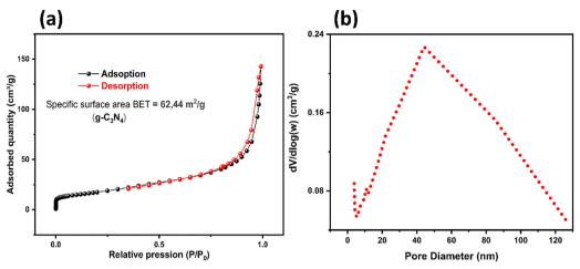
Fig. 7 BET isotherms (a) and pore-size distribution curve (b) of the g-C<sub>3</sub>N<sub>4</sub> support.
