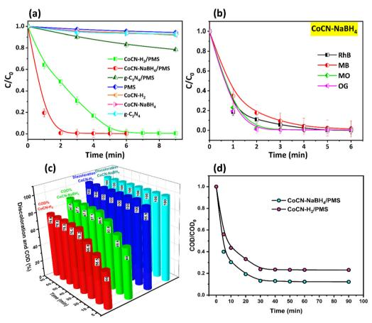
Fig. 8 (a) Removal rates of OG in various systems; (b) degradation of different pollutants using the CoCN-NaBH<sub>4</sub> catalyst; (c, d) COD removal of OG in the CoCN-x system.
