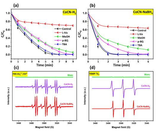
Fig. 10 Scavenger effect experiments on OG removal in (a) the CoCN $-H_2$ /PMS system, and (b) CoCN $-NaBH_4$ /PMS system, and EPR signals of different active free radicals (c) PBN $-SO_4^{\bullet-}/OH^{\bullet}$  and (d) TEMPO $^{-1}O_2$ .
