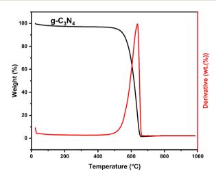
Fig. 1 TGA curve of g-C<sub>3</sub>N<sub>4</sub>.
