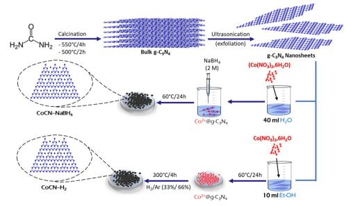
Scheme 1 Schematic diagram of chemical reduction pathways employed for CoCN-NaBH<sub>4</sub> and CoCN-H<sub>2</sub> preparation.
