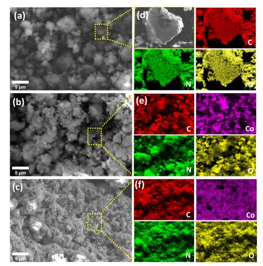
Fig. 5 SEM micrographs and EDS mapping of (a) and (d) g-C<sub>3</sub>N<sub>4</sub>, (b) and (e) CoCN-NaBH<sub>4</sub>, and (c) and (f) CoCN-H<sub>2</sub>
