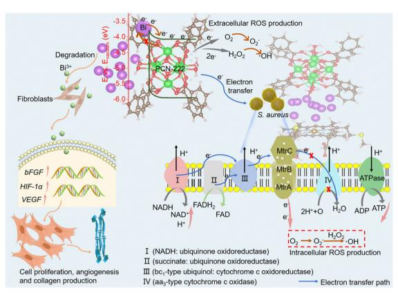
Fig. 4 Diagram illustrating the antibacterial mechanism and enhancement of cell proliferation and differentiation for accelerated wound healing. Reproduced with permission from ref. 56. Copyright 2023 American Chemical Society.
