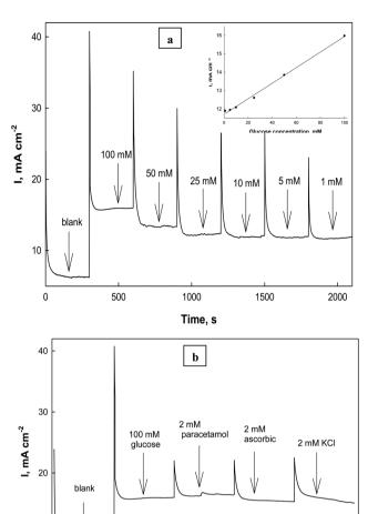
**Fig. 14** Chronoamperometry of electroxidation of glucose at 0.72 V in 0.5 M NaOH in the presence of (a) different concentrations of glucose from 1 mM to 100 mM, with the inset calibration plot and (b) different interfering species.
