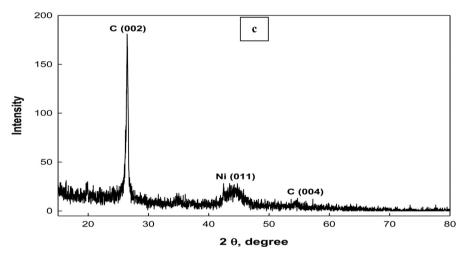
Fig. 4 (a) TEM, (b) SEM images, and (c) XRD pattern of the Ni(II)-SB/C complex
