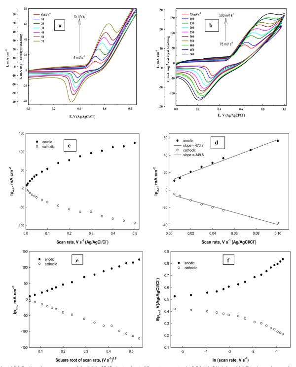
Fig. 9 (a) and (b) Cyclic voltammograms of the Ni(III) – SB/C electrode at different scan rates in 0.5 M NaOH. (c) and (d) The dependence of anodic (the solid dots) and cathodic (the open dots) peak currents on the scan rates. (e)  $I_{pa,c}$  vs. square root of scan rates and (f) dependence of peak potentials on the natural logarithm of the scan rates.
