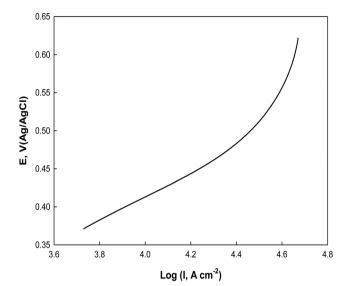
Fig. 13 Tafel line of Ni(ii)–SB/C in 0.5 M NaOH + 0.1 M glucose at 5 mV  $\rm s^{-1}.$
