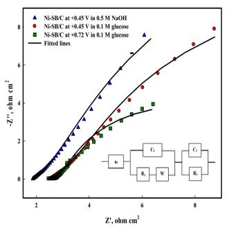
Fig. 15 Electrochemical impedance spectroscopy of Ni(III) –SB/C in 0.5 M NaOH and in the presence of 0.1 M glucose at +0.45 and 0.72V and the inset represents its equivalent circuit.
