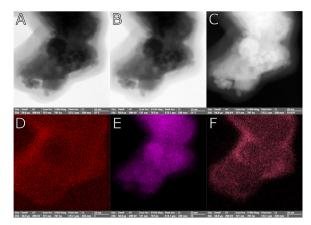
Fig. 2 STEM images of NG3 (5% GO) sample (A) brightfield, (B) darkfield, (C) high-angle annular dark-field imaging, and related element map (D) carbon (E) nickel (F) oxygen. Magnification: 760 000×, scale bar: 20 nm.
