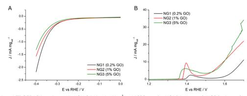
Fig. 8 (A) HER LSVs and (B) OER LSVs registered in KOH 0.1 M at 1 mV s<sup>-1</sup> and 1600 rpm for NG1 (black curve), NG2 (red curve) and NG3 (green curve) samples.
