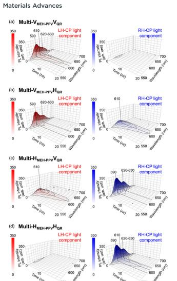
Fig. 6 Time-course changes in LH- (left) and RH- (right) CP light generated by (a) Multi-V<sub>MEH-PPV</sub>V<sub>QR</sub>, (b) Multi-V<sub>MEH-PPV</sub>H<sub>QR</sub>, (c) Multi-H<sub>MEH-PPV</sub>V<sub>QR</sub>, and (d) Multi-H<sub>MEH-PPV</sub>H<sub>OR</sub>. Red and blue indicate the light intensities of the LHand RH-CP components, respectively. Each convertor was excited by depolarized pulsed light at 470 nm.
