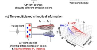
Fig. 1 Schematic illustration of (a) monochromatic and (b) multi-colored chiroptical information detected by steady-state PL spectroscopy, and (c) time-multiplexed chiroptical information detected by time-resolved PL spectroscopy.
