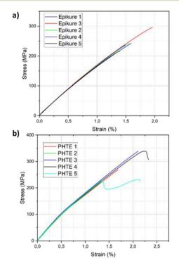
Fig. 4 Stress-strain curves obtained from the tensile test of (a) the Epikote-Epikure 04908-based composite and (b) the PHTE-Epikure 04908-based composite.
