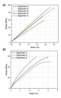
Fig. 3 Stress-strain curves of PHTE: (a) flexural testing of the resin and (b) tensile testing of the PHTE resin.
