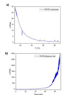
Fig. 1 (a) Viscosity profile of PHTE with increased temperature and (b) viscosity of the PHTE-Epikure mix at RT.
