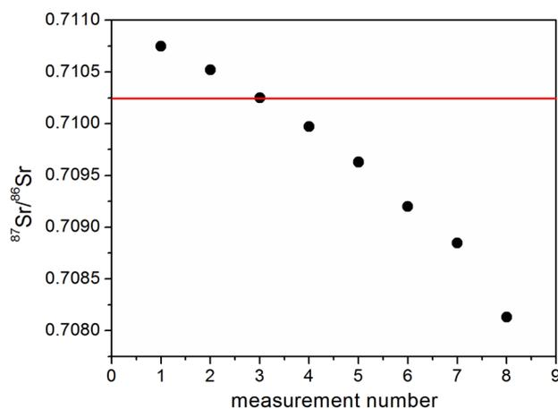
Fig. 1 Results for eight consecutive measurements of  $^{87}\text{Sr}/^{86}\text{Sr}$  isotope ratio using the  $^{93}\text{Nb}/^{89}\text{Y}$  pair as a calibrator. The SD values of individual replicates are smaller than the size of the dots. The red line represents the certified value.
