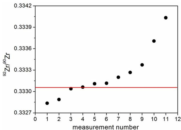
Fig. 2 Results for eleven consecutive measurements of  $^{92}\text{Zr}/^{90}\text{Zr}$  isotope ratio using the  $^{93}\text{Nb}/^{89}\text{Y}$  pair as a calibrator. The SD values of individual replicates are smaller than the size of the dots. The red line represents the certified value.
