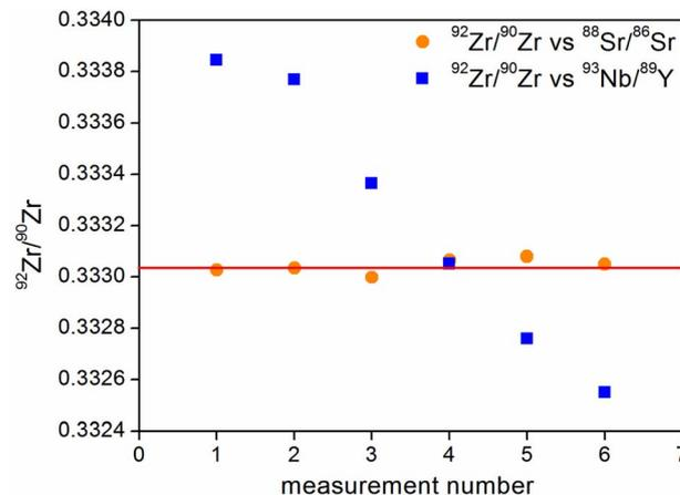
Fig. 4 Comparison of  $^{92}\text{Zr}/^{90}\text{Zr}$  isotope ratio determination using  $^{93}\text{Nb}/^{89}\text{Y}$  and  $^{88}\text{Sr}/^{86}\text{Sr}$  isotope pairs as calibrators. The SD values of individual replicates are smaller than the size of the dots. The red line represents the certified value.
