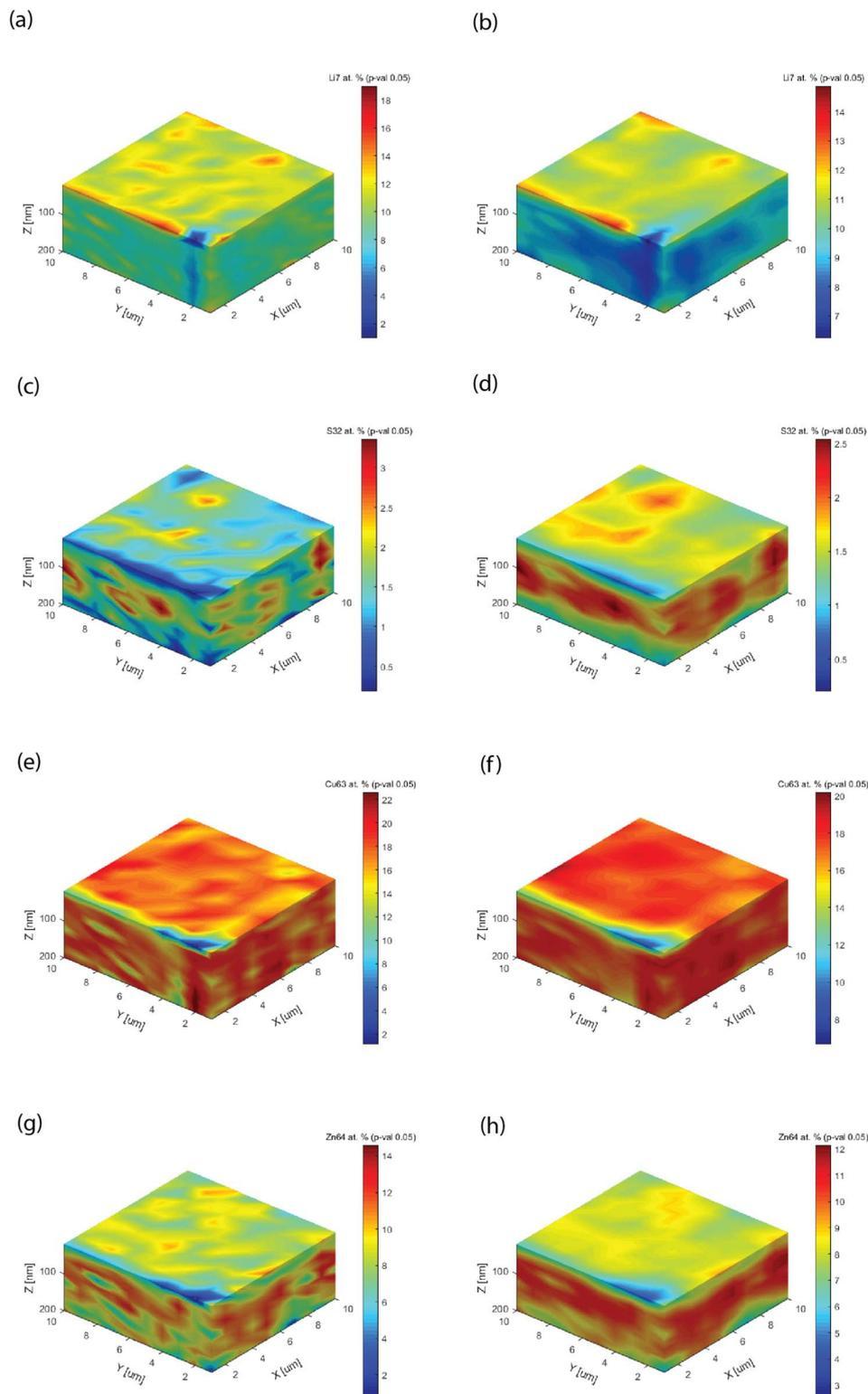
Fig. 7 Semi-quantitative concentrations for a selection of target analytes in the kesterite thin films obtained by HELDI mass spectrometry with two kernel sizes of  $k_1 = 1$  and  $k_2 = 3$ . The latter affects the spatial resolution of the elemental mappings. (a) Li7 ( $k_1$ ), (b) Li7 ( $k_2$ ), (c) S32 ( $k_1$ ), (d) S32 ( $k_2$ ), (e) Cu63 ( $k_1$ ), (f) Cu63 ( $k_2$ ), (g) Zn64 ( $k_1$ ), (h) Zn64 ( $k_2$ ).
