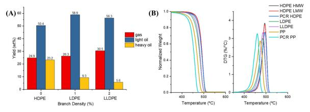
Fig. 2 (A) Yields of gas, light oil, and heavy oils of HDPE (no branch), LDPE (1% of branch), and LLDPE (2% of branch) from the fluidized bed laboratory pyrolysis reactor. (B) Thermal decomposition of HDPE HMW, HDPE LMW, PCR HDPE, LDPE, LLDPE, PP, and PCR PP analysed through TGA under  $N_2$  conditions (the same particle sizes as was fed to the fluidized bed reactor).
