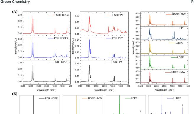
Fig. 1 (A) ATR-FTIR spectra of PCR HDPE, PCR PP and virgin polyolefins used in this study. (B) Zoomed-in quantitative 13C NMR results for PCR HDPE, HDPE HMW, LDPE, and LLDPE. The \* symbol is the tertiary carbon and 1 refers to the primary carbon, which indicates the end groups.
