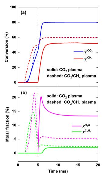
Fig. 7  $CO_2$  and  $CH_4$  conversion (a), as well as  $H_2O$  and  $C_2H_2$  molar fraction (b), as a function of time, for SEI = 140 kJ mol<sup>-1</sup>. The solid and dashed lines indicate the results for the  $CO_2$  plasma with post-plasma  $CH_4$  injection, and for the  $CO_2/CH_4$  plasma with post-plasma  $CO_2/CH_4$  injection, respectively. The vertical dashed line at 5 ms indicates the post-plasma mixing.
