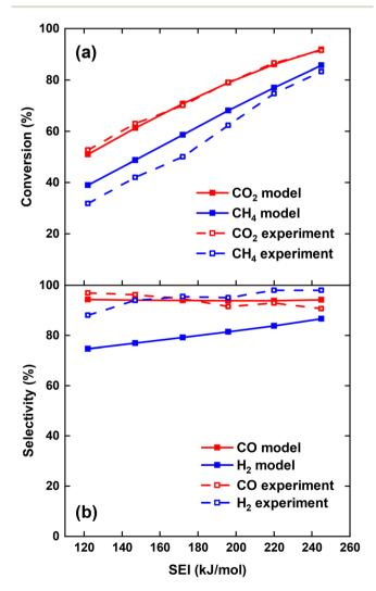
Fig. 1 Comparison of  $CO_2$  and  $CH_4$  conversion (a) and CO and  $H_2$  selectivity (b) between model and experiment, <sup>17</sup> as a function of the SEI.
