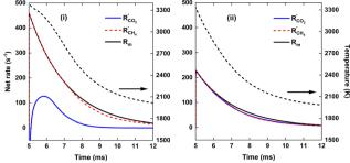
Fig. 10 Net rates of conversion of  $CO_2$  and  $CH_4$  and mixing rate (solid black line) as a function of time, for SEI = 220 kJ mol<sup>-1</sup> (left *y*-axis). The temperature is indicated by the dashed black line (right *y*-axis). The left panel (i) and right panel (ii) show the results for the  $CO_2$  plasma with post-plasma  $CH_4$  injection, and for the  $CO_2/CH_4$  plasma with post-plasma  $CO_2/CH_4$  injection, respectively.
