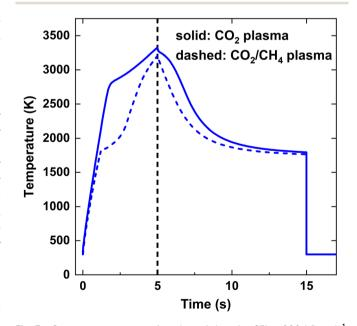
Fig. 3 Gas temperature as a function of time for SEI = 200 kJ  $mol^{-1}$ . The black vertical dashed line at t = 5 ms indicates the onset of post-plasma injection.
