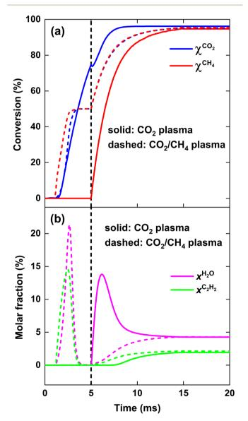
Fig. 9 CO<sub>2</sub> and CH<sub>4</sub> conversion (a), as well as H<sub>2</sub>O and C<sub>2</sub>H<sub>2</sub> molar fraction (b), as a function of time, for SEI = 220 kJ mol $^{-1}$ . The solid and dashed lines indicate the results for the CO<sub>2</sub> plasma with post-plasma CH<sub>4</sub> injection, and for the CO<sub>2</sub>/CH<sub>4</sub> plasma with post-plasma CO<sub>2</sub>/CH<sub>4</sub> injection, respectively. The vertical dashed line at 5 ms indicates the post-plasma mixing.
