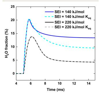
Fig. 12 H<sub>2</sub>O fraction as a function of time, for the CO<sub>2</sub> plasma with post-plasma  $CH_4$  injection, at  $SEI = 140 \text{ kJ mol}^{-1}$  and SEI = 220 kJmol<sup>-1</sup>. The dashed lines indicate the H<sub>2</sub>O fraction predicted by the WGS equilibrium.
