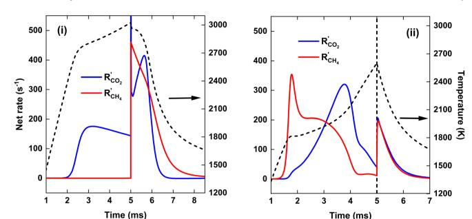
Fig. 8 Net rates of conversion of  $CO_2$  and  $CH_4$ , as a function of time, for  $SEI = 140 \text{ kJ mol}^{-1}$  (left y-axis). The temperature is indicated by the dashed black line (right y-axis). The left panel (i) and right panel (ii) show the results for the  $CO_2$  plasma with post-plasma  $CH_4$  injection, and for the  $CO_2/CH_4$  plasma with post-plasma  $CO_2/CH_4$  injection, respectively.
