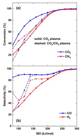
Fig. 5  $CO_2$  and  $CH_4$  conversion (a) and CO and  $H_2$  selectivity (b) as a function of the SEI. The solid and dashed lines indicate the results for the  $CO_2$  plasma with post-plasma  $CH_4$  injection, and for the  $CO_2/CH_4$  plasma with post-plasma  $CO_2/CH_4$  injection, respectively.
