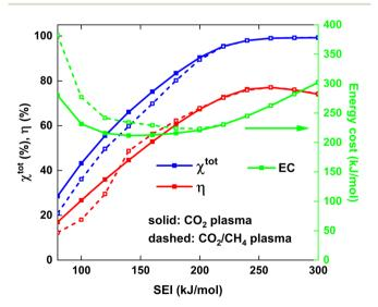
Fig. 6 Total conversion and ECE (left y-axis) and EC of conversion (right y-axis) as a function of the SEI. The solid and dashed lines indicate the results for the  $CO_2$  plasma with post-plasma  $CH_4$  injection, and for the  $CO_2/CH_4$  plasma with post-plasma  $CO_2/CH_4$  injection, respectively.
