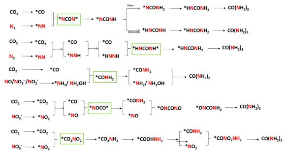
Fig. 10 Reaction pathways for the synthesis of urea by C-N coupling and its intermediates.
