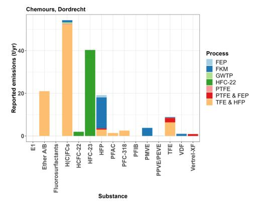
Fig. 4 Annual reported estimated emissions of fluorinated organic substances from Chemours, Dordrecht, to the air in 2021–2024. Colors represent different production processes. For the exact emission values, see ESI-2 Table S5.†
