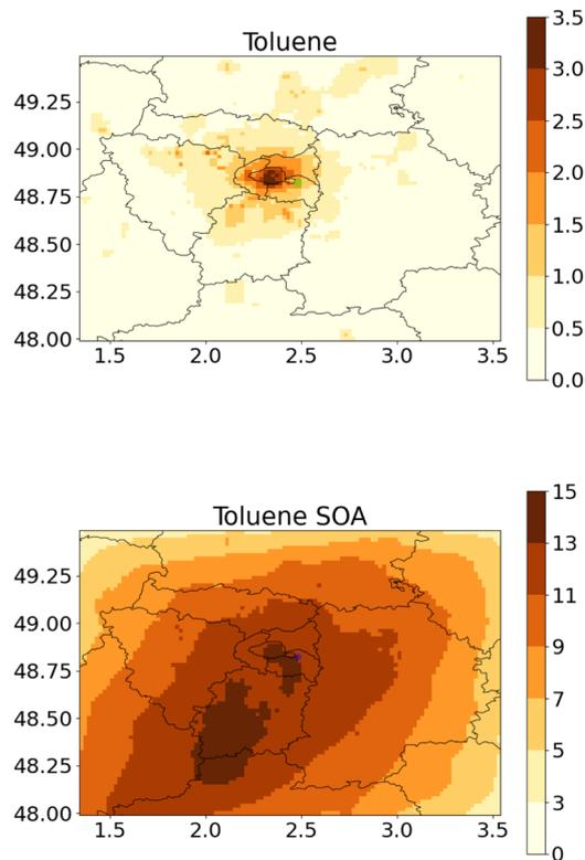
Fig. 2 Regional-scale toluene concentrations (left panel, in  $\mu\text{g m}^{-3}$ ) and toluene SOA concentrations (right panel, in  $\text{ng m}^{-3}$ ) simulated with the rdc. Mech. 3, in May–June 2014.
