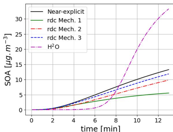
**Fig. 1** Toluene SOA concentrations (in μg m<sup>-3</sup>) simulated with different toluene SOA mechanisms (the near-explicit mechanism Mech. 2, the reduced mechanisms rdc. Mech. 1, rdc. Mech. 3 and H<sup>2</sup>O) for the flow tube experiment of Lannuque *et al.*<sup>39</sup>
