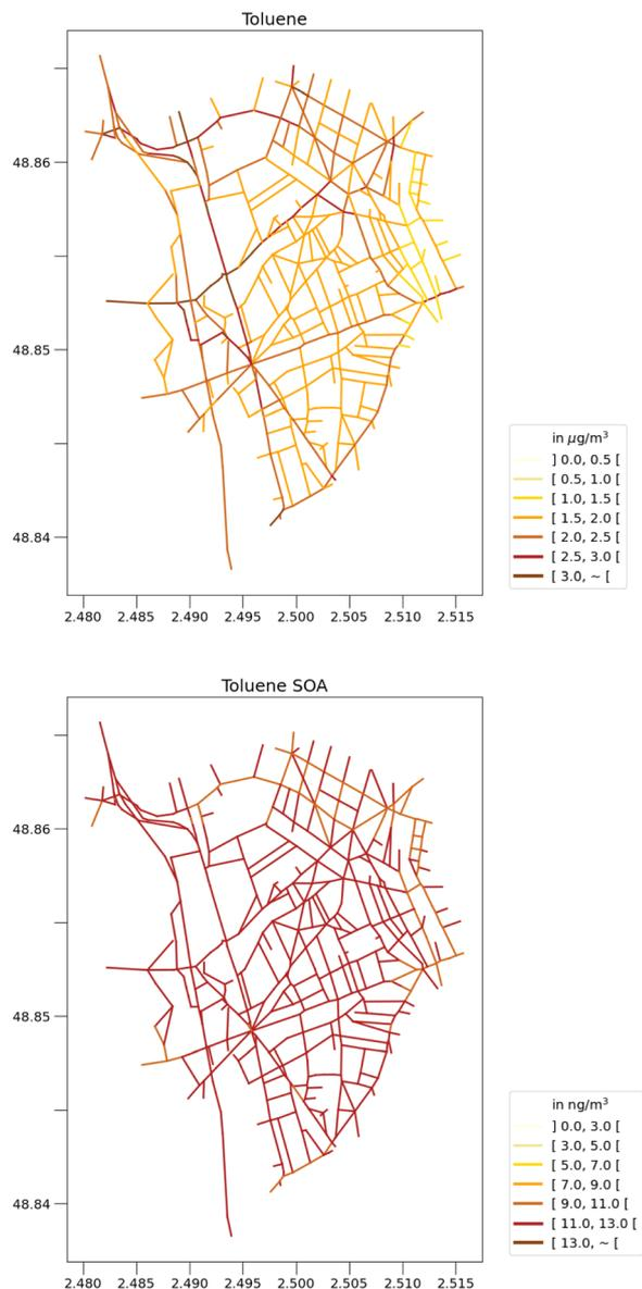
Fig. 3 Street-scale toluene concentrations (left panel, in  $\mu\text{g m}^{-3}$ ) and toluene SOA concentrations (right panel, in  $\text{ng m}^{-3}$ ) simulated with the rdc. Mech. 3, in May–June 2014.
