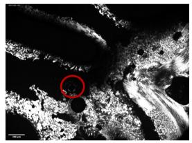
Fig. 6 Polarised-light microscope images of BTMAAOC at 5–10 °C, showing birefringence and a Maltese cross pattern (red circle) indicative of a lamellar liquid-crystalline phase. The images are taken at different points of the same sample slide with  $4 \times$  magnification.
