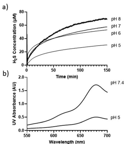
Fig. 1 (a)  $\text{H}_2\text{S}$  release profiles of **1** (50  $\mu\text{M}$ ) in different buffers. (b) Methylene blue UV-vis absorbance spectra of  $\text{H}_2\text{S}$  released from **1** as measured by the gas trapping method (1.5 mM **1** was incubated in buffers for 3 hours.  $\text{H}_2\text{S}$  gas was trapped by zinc acetate and measured by the methylene blue method).
