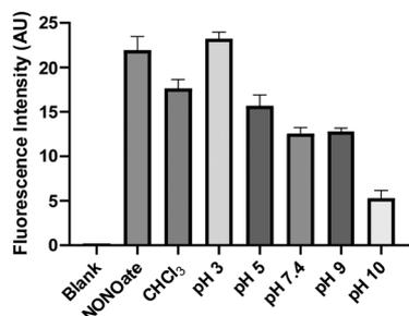
Fig. 4  $\text{NO}$  release from **2** measured by  $\text{NO}$  red. 6.4 mM **2** was incubated with  $\text{CHCl}_3$  or PBS buffers (containing 10% THF) for 1.5 h.  $\text{NO}$  was then trapped by  $\text{NO}$  red (40  $\mu\text{M}$ ), and its fluorescence ( $\lambda_{\text{em}}$  593 nm,  $\lambda_{\text{ex}}$  540 nm) was measured.
