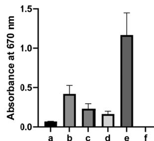
Fig. 2  $\text{H}_2\text{S}$  release from **6** measured by the gas trapping method. **6** (10 mM) or  $\text{Na}_2\text{S}$  (5 mM) was incubated in PBS buffer (pH 7.4) under various conditions.  $\text{H}_2\text{S}$  gas was trapped by zinc acetate and measured by the methylene blue method. (a) **6** only; (b) **6** with 20% HeLa cell lysate; (c) **6** with 10% plasma; (d) **6** with 20 mM cysteine; (e)  $\text{Na}_2\text{S}$  only; (f) blank.
