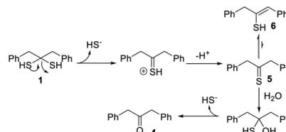
Scheme 3 The mechanism of  $\text{H}_2\text{S}$  release from **1**.
