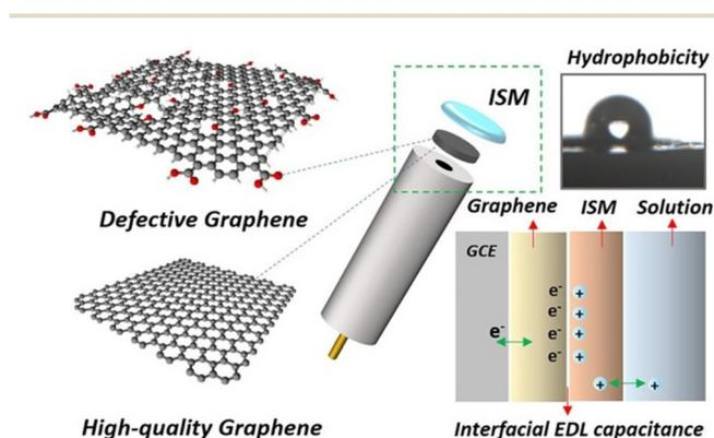
**Fig. 2** Graphical summary of defective and high-quality graphene used as the solid contact material in an ISE, along with a photograph of the contact angle of water on reduced graphene oxide, and a schematic figure of the interfacial EDL capacitance of ISE.<sup>86</sup> Copyright 2021, Elsevier.
