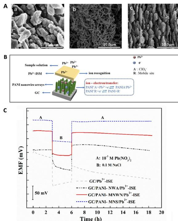
**Fig. 6** (A) SEM images of PANI-NWA (a), PANI-MNWN (b), and PANI-MNS (c) deposited on a glassy carbon electrode by direct electro-deposition. (B) Sensing mechanism for a NWA-based ISE. (C) Potential curves of different  $\text{Pb}^{2+}$ -ISEs in  $10^{-3} \text{ M Pb}(\text{NO}_3)_2$  for 3 h,  $0.1 \text{ M NaCl}$  for 3 h, and then  $10^{-3} \text{ M Pb}(\text{NO}_3)_2$  again for 12.5 h.<sup>166</sup> Copyright 2021, Elsevier.
