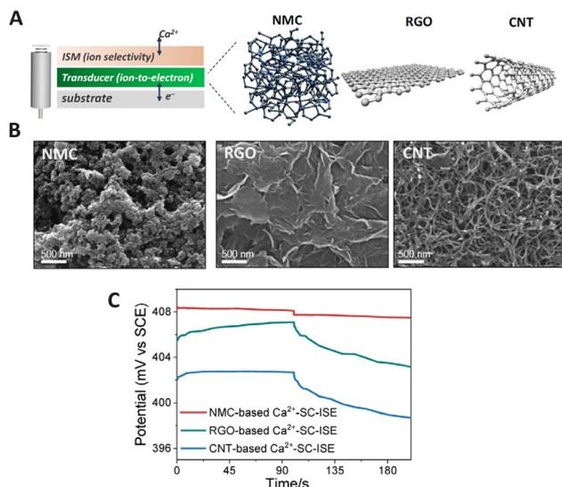
**Fig. 3** (A) Schematic diagram of SC-ISEs based on NMC, RGO, and CNTs. (B) SEM images of NMC, RGO, and CNTs. (C) Chronopotentiometric curves obtained for the NMC-based, RGO-based, and CNT-based SC-ISEs for the detection of Ca<sup>2+</sup>.<sup>96</sup> Copyright 2022, MDPI.
