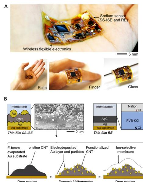
**Fig. 9** (A) Overview of a wireless all-in-one sodium sensor with a solid-state ISE (SS-ISE) and a reference electrode (RF), attached to different substrates. (B) Graphical depiction of the SS-ISE and RF, and the production steps for the SS-ISE.<sup>179</sup> Copyright 2021, Elsevier.
