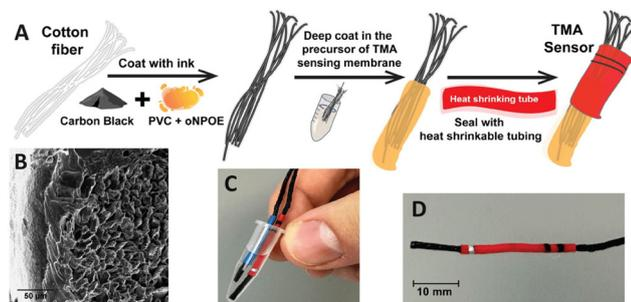
**Fig. 4** (A) The process of preparing a home-made TMA sensor for vaginosis analysis. (B) A SEM cross-section image of the membrane coated TMA sensor (scale bar is 50 μm). (C and D) Photographs of the sensor depicting its portability and size.<sup>102</sup> Copyright 2023, MDPI.
