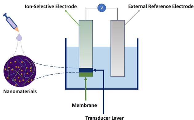
Fig. 1 A schematic representation of a typical nanomaterial-based SC-ISE.
