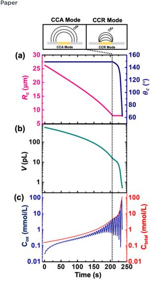
Fig. 5 (a) Contact radius (left Y axis) and contact angle (right Y axis) used for the simulation of a DCE droplet dissolution in (b) simulated volume of the droplet as a function of time. (c) Simulated concentration of  $(Cp^*)_2$  Fe<sup>III</sup> (left axis) denoted as  $C_{\rm ox}$  and total concentration of redox active species (right axis) denoted as  $C_{\rm total}$  during the dissolution of the droplet. The vertical dotted line represents the transition from CCA to CCR mode.
