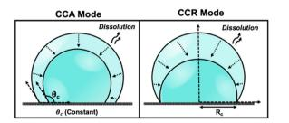
Fig. 1 Schematic depicting various modes of droplet dissolution: Constant Contact Radius Mode (CCR) and Constant Contact Angle Mode (CCA).
