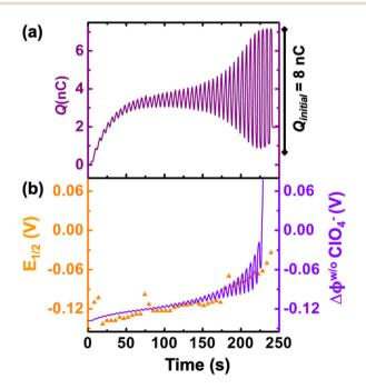
Fig. 6 (a) Charge obtained by integrating the area under the experimental cyclic voltammograms. (b) experimental half-wave potential  $(E_{1/2}$ , shown in orange) and simulated apparent standard potential corrected from the junction potential loss  $(E^{\circ}$ , shown in violet) during the course of the droplet dissolution.
