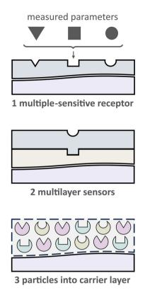
Fig. 5 Schematic of the three most common designs for creating multiparameter optical sensors via different recognition options: (1) multiple-sensitive receptor, (2) multilayer sensors, (3) (nano)particles into carrier laver.
