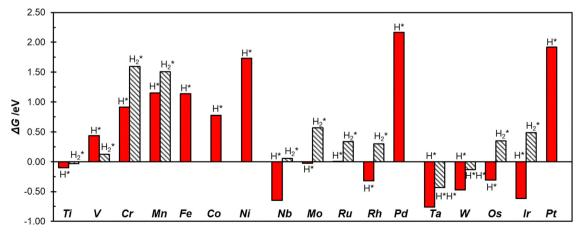
Fig. 3 Gibbs free energies of H\* and H<sub>2</sub>\*/H\*H\* intermediates adsorbed at TM@COF SACs.
