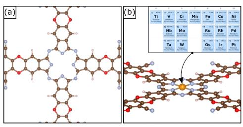
Fig. 1 (a) Top view of the selected COF and (b) example of the TM@COF structure. Inset: TMs selected for this study. Oxygen (red), carbon (brown), nitrogen (light blue) and hydrogen (white). The generic metal atom in (b) is indicated in orange
