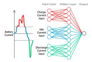
Fig. 5 Illustration of the assembly of the load-classification of neutral network with presentation of the input data divided into three subsets based on the three types of battery behaviour (charging, idling, and discharging) segregated by three different colours. Reproduced with permission from ref. 84. Copyright 2016, Elsevier.
