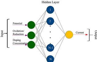
Fig. 6 Illustrative setup of the input, hidden, and output layers in ANN modelling for the prediction of performance behaviour of CoCeO<sub>2</sub>/rGO nanocomposite supercapacitors. Reproduced with permission from ref. 105. Copyright 2018, the American Chemical Society.
