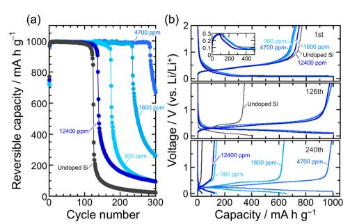
Fig. 4 (a) Variation in discharge (Li-extraction) capacity of Si electrodes in 1 M LiPF<sub>6</sub>/EC:DEC with 5 vol% FEC versus number of cycles at a fixed Li-insertion level of 1000 mA h  $g^{-1}$ . (b) Charge/discharge curves of the Si electrodes at the first, 126th, and 240th cycles. Inset: enlarged view of the first charge-discharge curves of Si-based electrodes.
