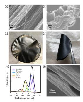
Fig. 1 Surface morphology of the prepared materials. (a) SEM image of SWMCNT, (b) SEM image of Ox-SWCNTs. (c and d) Optical image of the free-standing film of GO/Ox-SWCNT, (e) C 1s XPS spectra of GO/ Ox-SWCNT, and (f) cross section SEM images of GO/Ox-SWCNT.
