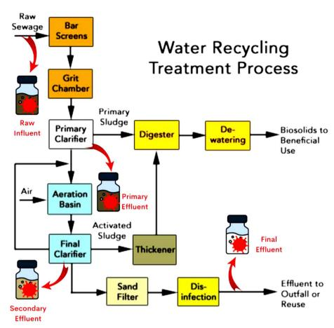
Steven M. Clouse WRC activated sludge treatment process stages and sample collection points.
