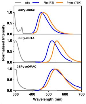
Fig. 2 UV-Vis absorption, fluorescence (RT), and phosphorescence (77 K) spectra of 3BPy-mDCz, 3BPy-mDTA, and 3BPy-mDMAC respectively in toluene (Tol)  $(1 \times 10^{-5} \text{ M})$ .
