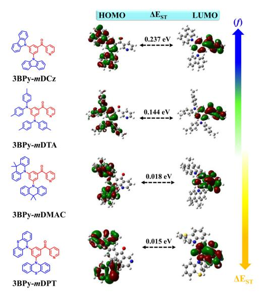
Fig. 1 The distribution of the molecular orbital of the HOMO and LUMO with a calculated  $S_1$  and  $T_1$  energy gap ( $\Delta E_{ST}$ ). The right side top and bottom of the arrow marks indicate the enhancement of oscillator strengths (f) and reduction of  $\Delta E_{ST}$  when increasing the donor strength
