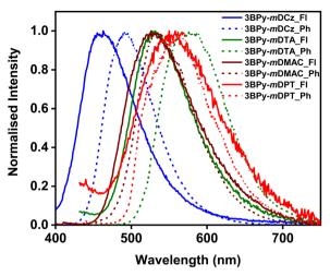
Fig. 3 Fluorescence (Fl) and phosphorescence (Ph) spectra of 7 wt% **3BPy-mDCz**:DPEPO, **3BPy-mDTA**:mCBP, **3BPy-mDMAC**:mCBP 3BPy-mDPT:mCBP doped film.
