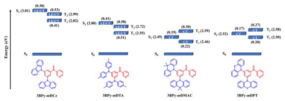
Fig. 6 Energy level diagram of excited states (S<sub>1</sub>, T<sub>1</sub> and T<sub>2</sub>) for **3BPy-mDCz**, **3BPy-mDTA**, **3BPy-mDMAC** and **3BPy-mDPT** where the value in brackets indicates the hole–electron overlap for the specified level.
