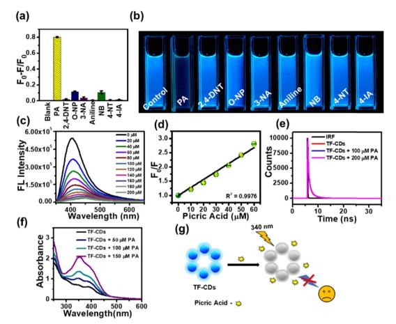
Fig. 3 (a) Selectivity of TF-CDs towards various NACs, (b) photographs of TF-CDs in the presence of various NACs captured under UV light, (c) FL spectra of TF-CDs after adding different concentrations of PA (0–200  $\mu$ M) and (d) relationship between PA concentration vs.  $F/F_0$  for TF-CDs. (e) Lifetime data and (f) UV-vis spectra of TF-CDs for different concentrations of PA. (g) Schematic representation of quenching of TF-CDs after the addition of PA.
