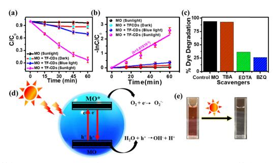
Fig. 6 (a) and (b) Comparative photodegradation of MO under blue light and sunlight and their rate, respectively, (c) effect of scavengers on the degradation of MO, (d) possible mechanism for MO degradation by TF-CDs, and (e) images of MO before and after sunlight exposure (after degradation).
