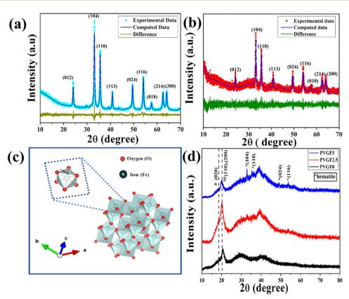
Fig. 1 (a) and (b) Experimental and computed XRD patterns of natural  $\alpha$ -hematite and Gd-incorporated  $\alpha$ -hematite, respectively. (c) Unit cells of Gdincorporated  $\alpha$ -hematite. (d) XRD patterns of natural Gd-incorporated  $\alpha$ -hematite nanocomposite membranes suggesting that incorporation of nanocomposite into the polymer matrix enhances the polar phase, finding a maximum in PVGF2.5.
