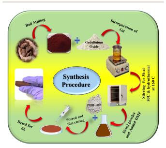
Scheme 1 Schematic representation of the synthesis procedure.
