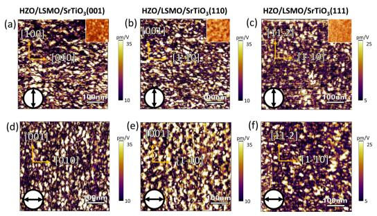
Fig. 5 (a-c) PFM in-plane amplitude images for the HZO films on LSMO/SrTiO<sub>3</sub>(001), LSMO/SrTiO<sub>3</sub>(110), and LSMO/SrTiO<sub>3</sub>(111), respectively. Response is probed along the vertical direction as indicated in the bottom-left. Top-right insets show the topography images. (d-f) Idem, while probing along the horizontal direction.
