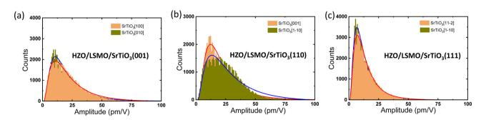
Fig. 6 (a-c) Histograms of the PFM out-of-plane amplitude images for the three HZO films grown on LSMO/SrTiO<sub>3</sub>(001), LSMO/SrTiO<sub>3</sub>(110), and LSMO/ SrTiO<sub>3</sub>(111), respectively, along the indicated directions. The line above the histogram corresponds to lognormal fitting
