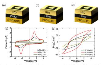
Fig. 2 (a-c) Sketch of HZO films grown on LSMO/SrTiO<sub>3</sub>(001), LSMO/ SrTiO<sub>3</sub>(110), and LSMO/SrTiO<sub>3</sub>(111), respectively. (d and e) Corresponding I-V and P-V loops measured at 1 kHz for the three samples.
