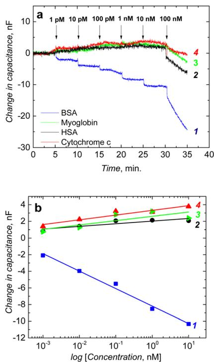
**Fig. 6** (a) Measurement of the change in the capacitance of the semi-covalently surface imprinted macroporous MIP film in the presence of (1) BSA, (2) HSA, (3) myoglobin, and (4) cytochrome c before post-imprinting modification and (b) corresponding calibration curves. Measurement was performed in 10 mM MES buffer (pH = 4.2). Potential: 0.2 V; frequency: 10 Hz.
