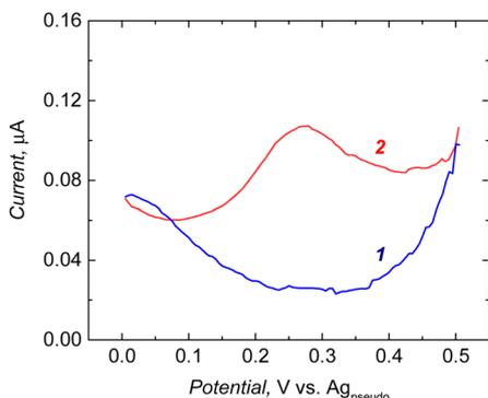
**Fig. 1** Electrochemical measurement performed at the electrode coated with 3,3'-bithiophene (**CR2**) and *p*-bis(2,2'-bithien-5-yl)methylbenzoic acid (**FM2**) co-polymers (1) before and (2) after its modification with aminoferrocene. DPV measurement conditions: pulse height: 2.5 mV, pulse width: 100 ms, step height: 5 mV, step time 500 ms, 0.1 M LiClO<sub>4</sub>/ACN.
