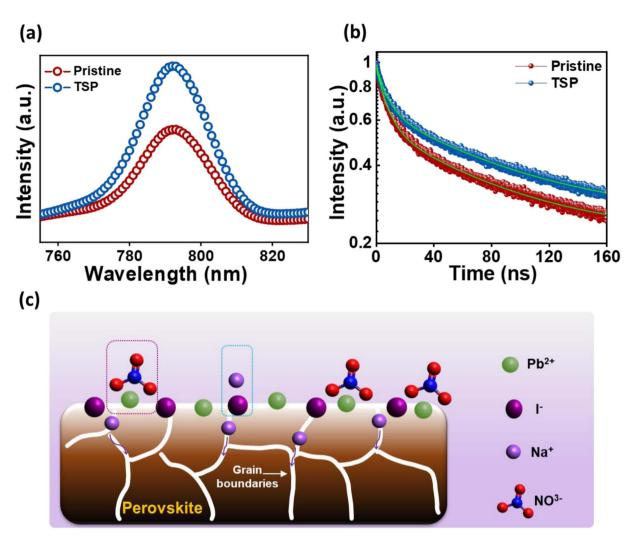
Fig. 4 (a) PL spectra for pristine and TSP films. (b) TRPL spectra for pristine and TSP films. (c) Probable mechanism for interaction of NaNO $_3$  at the perovskite/ETL interface.
