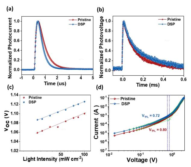
Fig. 6 (a) Transient photocurrent (TPC) and (b) transient photovoltage (TPV) of pristine and DSP devices, (c)  $V_{OC}$  versus light intensity of the devices for pristine and DSP devices and (d) SCLC measurements of hole-only devices for pristine and DSP devices.
