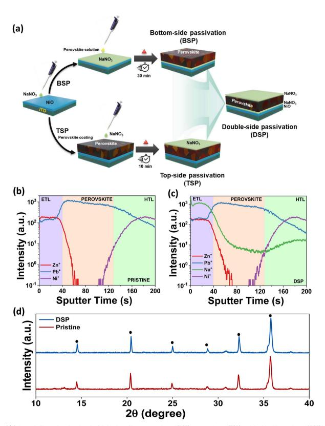
Fig. 1 (a) Schematic illustration showing the fabrication of bottom passivated (BSP), top passivated (TSP) and double side passivated (DSP) layers. TOF-SIMS depth profiles (from surface to bottom) of perovskite films: (b) pristine and (c) DSP films. (d) XRD patterns for perovskite films for pristine and DSP perovskite layers.
