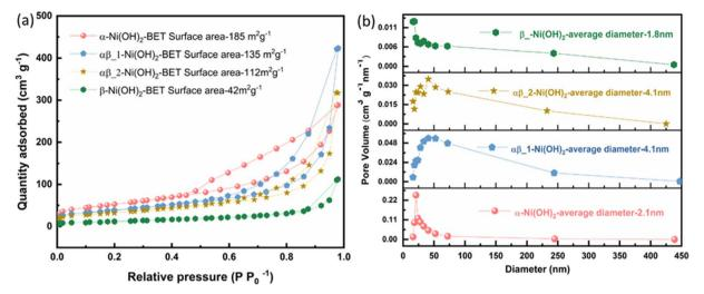
Fig. 3 (a) Nitrogen adsorption-desorption isotherm of different phases of nickel hydroxide (b) pore size distribution based on the BJH model of different phases of nickel hydroxide.
