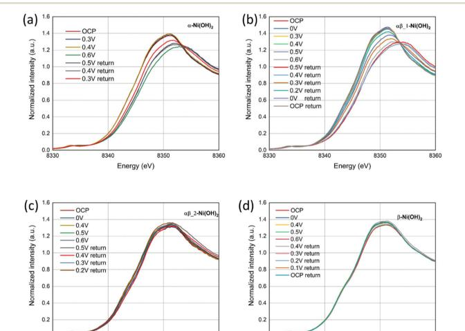
Fig. 9 In situ Ni K-edge XANES spectra of (a)  $\alpha$ -Ni(OH)<sub>2</sub>, (b)  $\alpha\beta$ \_1-Ni(OH)<sub>2</sub>, (c)  $\alpha\beta$ \_2-Ni(OH)<sub>2</sub> and (d)  $\beta$ -Ni(OH)<sub>2</sub> under a oxidation and reduction scans.
